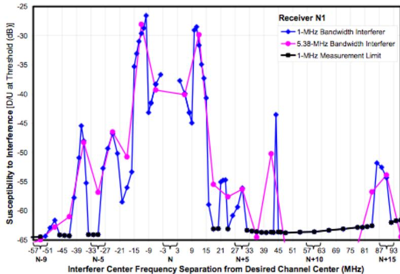
Figure 7-1. D/U With 1-MHz Undesired Signal Bandwidth
