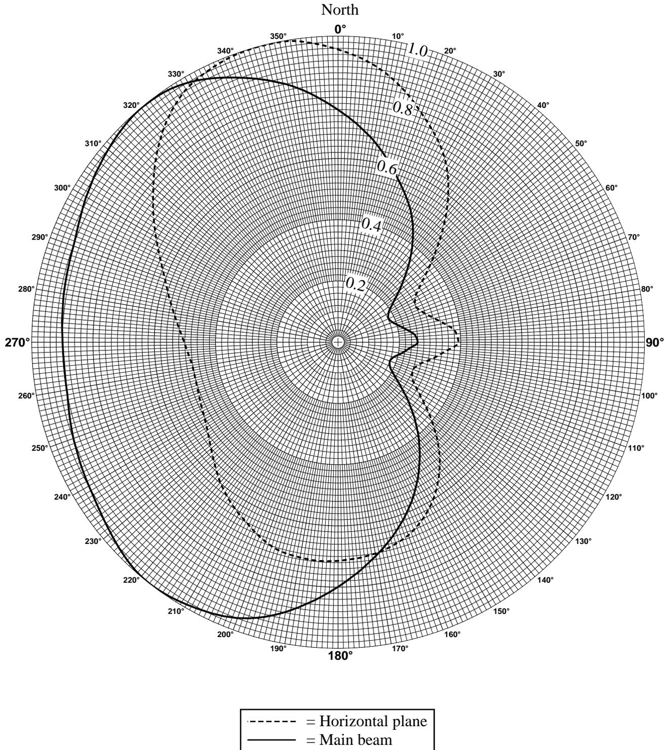
Comparison of Main Beam and Horizontal Plane Azimuth Patterns
